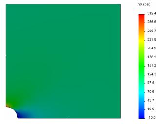
The analytical value for the maximum normal stress is  $\sigma_{\text{max}}$ = 302.452 psi.
