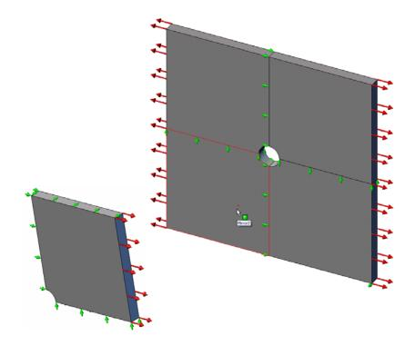
You will calculate the stresses of a 20 in x 20 in x 1 in square plate with a 1 inch radius hole at its center. The plate is subjected to a 100 psi tensile pressure.
