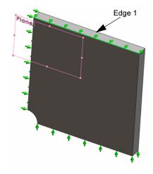
After applying all fixtures, three items: (Symmetry-1) and (Reference Geometry-1) appear in the Fixtures folder.
