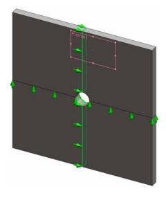
To prevent displacement of the model in the global Z-direction, a fixture on the vertex shown in the figure below must be defined.
