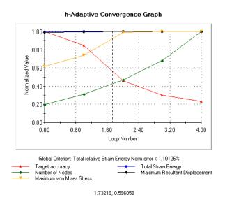
**Note:** To further improve the accuracy of the solution, it is possible to continue with the h-adaptivity iterations by initiating subsequent study runs. Each subsequent study run uses the final mesh from the last iteration of the previous run as the initial mesh for the new run. To try this **Run** the H-adaptive study again.
