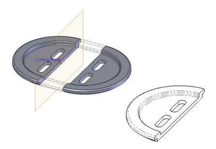
4 Create a section view from the Top view. Click **Section View** (1) on the Drawing toolbar or the **View Layout** tab of the Command Manager.
