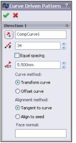
**Note:** Each instance of the extrusion was 6 mm wide but we patterned it with a spacing of 5.5 mm. This makes sure that the final pattern does not have gaps when it makes the turn up the slope at the end of the Binding Base Plate.
