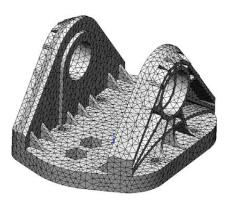
2 Type **4.0mm** for the mesh element size. This will create smaller elements.
