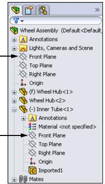
7 Check the assembly. The Inner Tube should be correctly positioned on the Wheel Hub with the Tube Stem coming through the hole in the Wheel Hub.
