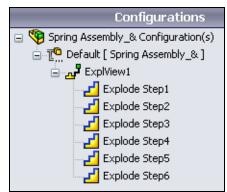
When using **Explode** or **Collapse**, all parts move from their collapsed position *directly* to their explode position regardless of the steps taken to get from collapse to explode.
