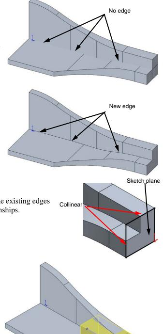
24 Create a **20mm** fillet to fill in the area behind the last extrusion.
