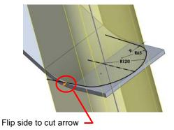
16 To change the side to remove, you can click on the Flip Side To Cut arrow or select Flip side to cut in the PropertyManager.
