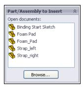
5 Click on the Origin. This will insert the part Strap\_right on the assembly Origin with its three planes aligned to the corresponding planes in the assembly.
