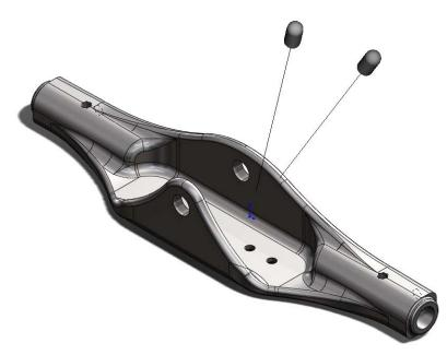
**3** Double-click light Directional<sup>2</sup>. The position of the light can be changed by dragging the manipulator or by the sliders and entry boxes in the PropertyManager.
