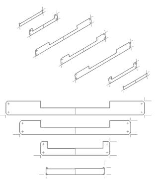
3 Select each sketch in order at the point indicated. You do not have to pick on an exact point. The idea is that where we select is close to the intersection of the horizontal and vertical lines.
