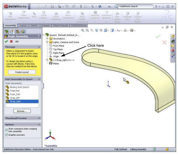
6 Click Insert, Component, Existing Part/Assembly from the menu and insert the Strap\_left and Foam\_Pad\_curved part using the same method.
