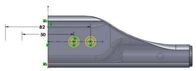
12 Click 🗹 . The two holes are correctly created an placed on the part.
