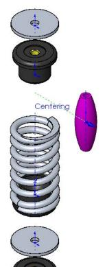
**15** Click on the Spring Dampener, then drag it by the green arrow of the **Triad** until it is alongside the Spring.
