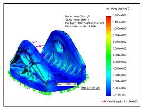
6 The FOS is 1.2 which is less then with the courser mesh. As the maximum stress was higher, the actual FOS is lower than before.
