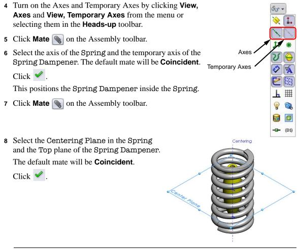
**Note:** Normally, mates are added to reflect the mechanical conditions of the assembly. In some cases, such as the Spring Dampener, the part may float in the actual assembly. The Spring Dampener can move along the axis as it will be held by bolts at either end. Because we want to contain the Spring Dampener in our model we use reference geometry to hold it in position.
