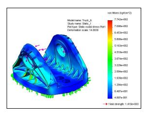
**10** The Design Check plot shows a minimum factor of safety of 1.8.
