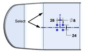
Notice that the Sketch is not fully defined. To determine what's wrong, try to drag the right end of the horizontal centerline.
