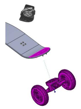
8 Click **Re-use Sub-assembly Explode**. This explodes a sub-assembly of the sub-assembly.
