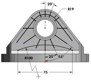
6 Create ribs. Use the rib tool to create ribs that are **2mm** thick and have **2°** of draft.
