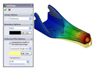
Adjust the transparency slider to be able to see the undeformed shape.
