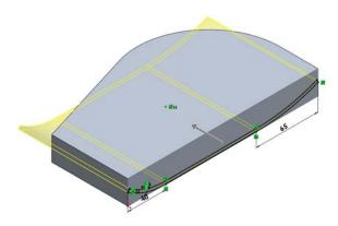
21 Select **Flip side to cut**. Now the cut will keep the material that is inside the sketch and remove the material that is outside the sketch.
