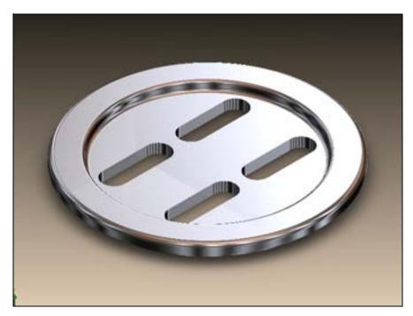
□ This part is the center anchor for each of the two bindings. The Mountainboard uses two of these parts, one for each binding.
