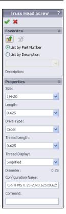
21 Use Toolbox to add 8 - 32 x 1.125 inch Truss Head Screws and 8 - 32 Machine Screw Nut Hex to the eight locations to hold the Truck to the Deck.
