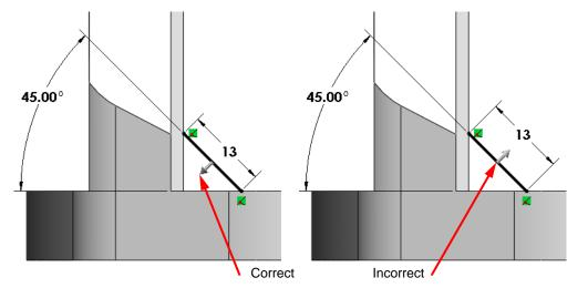
9 Click . The Rib tool creates an extrusion that fills in material up to the next geometry it encounters.
