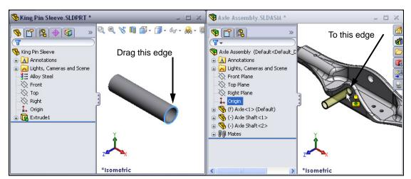
10 Press the **Tab** key to reverse the orientation of the mates. When the cursor shows the **Pin in Hole** and the orientation is correct, drop the King Pin Sleeve. It will receive both a **Concentric** and **Coincident** mate.
