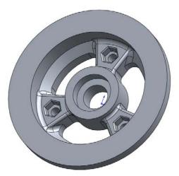
12 Add additional fillets to round remaining sharp edges. Add a 3 mm fillet. Select the face and edges shown. When you select a face, all edges of that face will be filleted.
