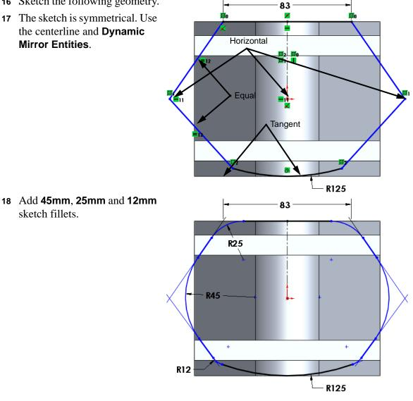
Note: When you add the first of each pair of fillets, you will get a warning that "At least one segment being filleted has a midpoint or equal length relation. Geometry may have to move to satisfy this relation when the fillet is created. Do you want to continue?"
