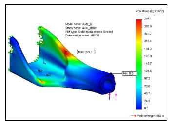
4 There is a plot title in the upper left corner of the graphics area. Notice that the deformation scale is 103.087. This means that we are seeing slightly more than 100 times the actual deformation of the part. This is done just to make it easier to visualize the result.
