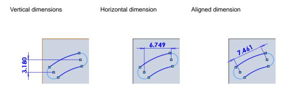
To lock in the dimension alignment you want, click the right mouse button to set it. The cursor  $\overline{k}$  shows that clicking the right mouse button will lock the alignment. Once the dimension alignment is locked, the cursor changes to  $\overline{k}$ , to show that you can now unlock the dimension alignment by clicking the right mouse button. Once locked, the alignment of the dimension will stay active no matter where you then move the cursor.
