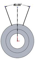
Start the arc at the origin and drag it to the top end of one of the lines. Release the mouse button, then press the left mouse button again and drag to the top of the other line.
