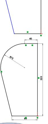
**19** Create a **Blind** extrusion to a depth of **25mm**.
