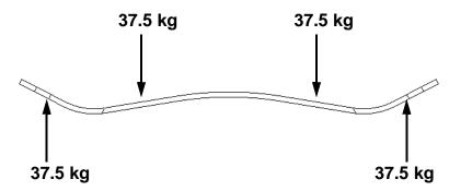
How do the results change when the rider's weight is not symmetrical? If the rider puts all his weight on one foot then  $F_1 = 75$  kg and  $F_2 = 0$ . How do we determine  $F_3$  and  $F_4$  since they are no longer equal?
