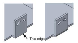
The profile of the tab shows that the thickness is no longer uniform. We must add a fillet to the inside edge of the tab at the correct radius to keep the material uniform.
