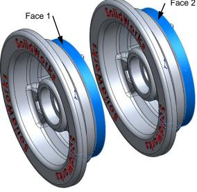
9 Reverse the alignment. The two cylindrical faces can be concentric in two orientations. The initial orientation is based on which of the two possibilities is closest. Press the Tab key. This will toggle the two possible alignments.
