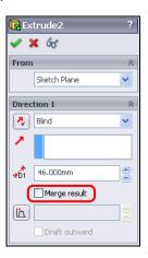
9 Examine the results. The FeatureManager design tree shows two solid bodies. Because the results of the two extrusions were not merged, each remains separate.
