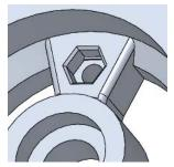
To allow the fillets to be added to the pattern, we must roll back the model to before the circular pattern.
