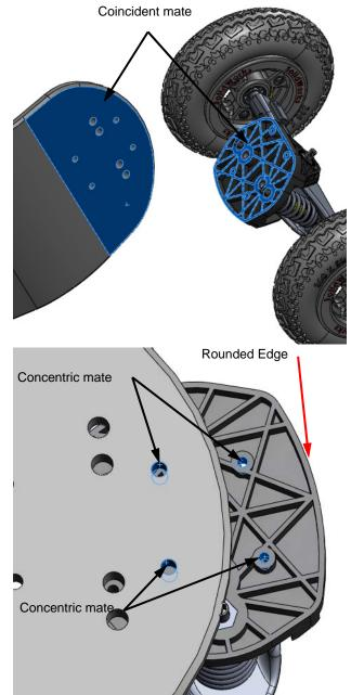
3 Add Concentric mates between the two holes in the Truck and the corresponding holes in the Deck.
