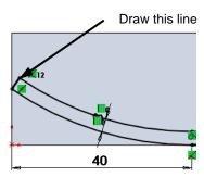
12 If the line does not become fully defined, add a relationship to make the line perpendicular to the arc. Because we cannot add a perpendicular relationship between the arc itself and the line we will add a coincident relationship between the line and the centerpoint of the are. By basic geometry this will make the line perpendicular to the arc.
