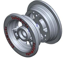
**13** Mate an Index Pin to the corresponding Index Hole. Click
