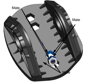
10 Insert three more instances of the 8mm Threaded Insert into the assembly and mate them to the three remaining hex holes.
