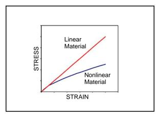
Using a linear material model, the maximum stress magnitude is not limited to yield or to ultimate stress as it is in real life.
