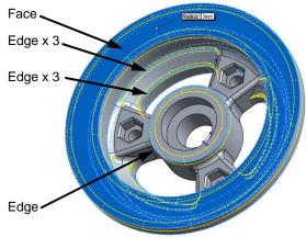
**13** Finish the front by adding a 0.5 mm by 45 degree chamfer to edge of the hole where the bearing will be inserted.
