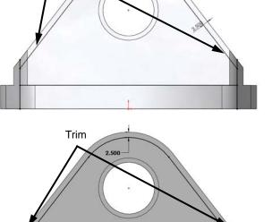
**10** Create an additional 2.5mm offset from Offset this edge the edge of the circular cutout. This will be used to hold the bearing.
