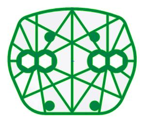
Examine the ribs. Notice that with the exception of the center vertical rib, all the remaining ribs radiate from a single point between the hex holes on each side.
