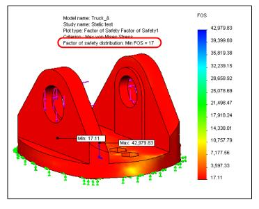
the stress in the vertical bosses is transmitted to the base plate.
