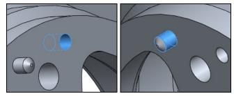
**Note:** Check to make sure that the hole for the Tube Stem lines up on the two Wheel Hubs. If it does not, edit the last mate and change the mate to the correct hole.
