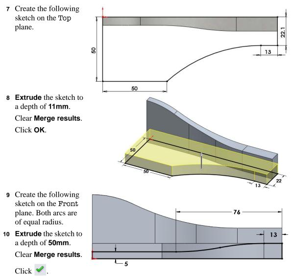
11 Examine the Solid Bodies folder. There are now three solid bodies. We will combine all the bodies to make a single solid, however we need to do it in two steps. First, Boss-Extrude3 and Boss-Extrude4 will be combined to get the common volume. This is the same as was done with Extrude1 and Extrude2. Next, the two combined volumes will be added together.
