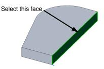
When you are over the edge, the cursor feedback will be  $\searrow_{\varkappa}$ . This is the feedback for coincident, meaning you are on the edge. Sketch a line to the right.
