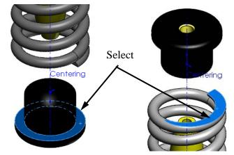
15 Add another Spring Retainer to the assembly. Hold the **Control** key and drag the Spring Retainer from the FeatureManager design tree into the graphics area
