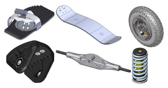
We will first put together all the sub-assemblies that make up the wheel assemblies. Then we will add the wheel assemblies and bindings to the deck to complete the mountainboard.
