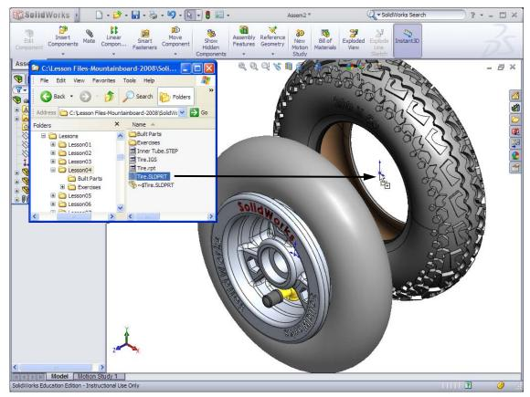
4 Add mates between the three principal planes of the Tire and the assembly just like we did for the inner tube.
