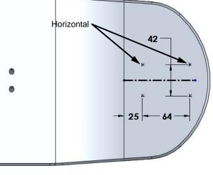
6 Click **OK** in the **Hole Wizard** dialog. These are the four holes that will be used to mount the Truck.
