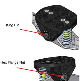
Add, from Toolbox, two B18.3.5M 4x0.7x10 Socket FCHS-10N screws to hold the bottom of the spring assemblies to the axle.
