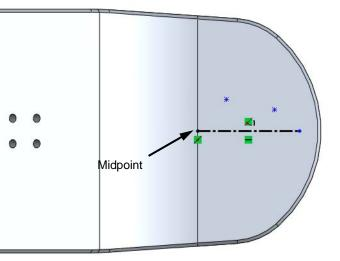
5 Dimension the points as shown. Add a Horizontal relationship between two points as shown.
