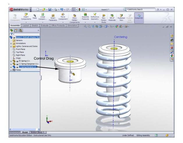
16 Mate the second Spring Retainer to the Centering axis of the Spring and the top ground face, just as was done to the first Spring Retainer.
