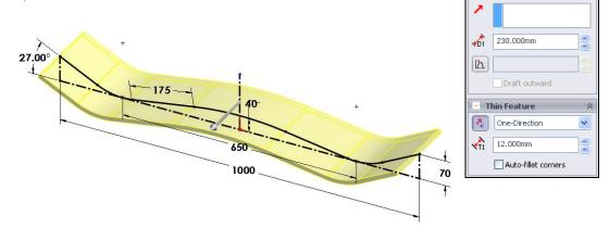
Because we are extruding an open sketch, **Thin Feature** is checked by default. For thin features, **T1** is the thickness of the extrusion in the sketch plane. Thickness can be added to either side of the sketch or both. Type **12mm** for the thickness.
