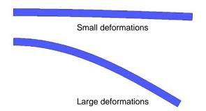
The preceding figure shows a cantilever beam in bending with small deformations and large deformations.
