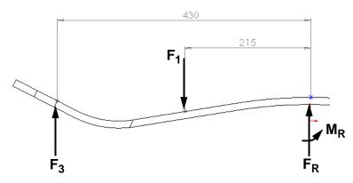
At this point in the model,  $F_{R} = F_{1} - F_{3} = 75 - 56.25 = 18.75$  kg.
