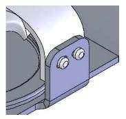
context of an assembly allows you to take advantage of geometry and dimensions of other components while creating matching or related features. Using geometry outside the part creates **External References** and **In-context Features**.
