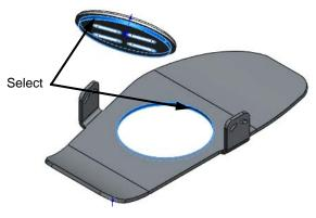
**Note:** The Binding Anchor has been rotated in the graphic to make it easier to see the two faces. You will have to rotate the model to be able to select both faces.
