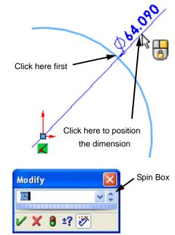
6 Input the dimension by typing 82 in the Spin Box. Click ✓ to accept the dimension.
