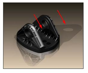
Without shadows, the relative position between model and the surface may be difficult to understand. The model may look like it is sitting on the surface, but without shadows you can't tell. Adding shadows may show that the part is actually floating above the surface.
