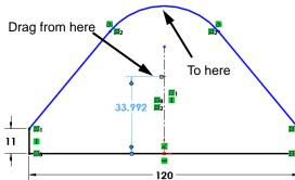
6 Once the dimension goes to the top of the arc, it can be changed to the correct value of **72mm**.
