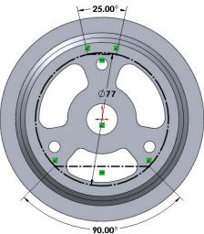
6 Add angular dimensions. To fully define the construction geometry add the angle dimensions show. Select the Smart Dimension tool ?, then select the Origin and each end of a line. Drag the dimension to the position shown. Repeat for the other dimension.
