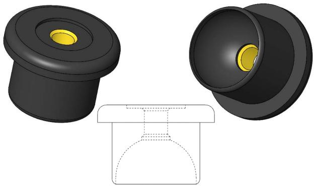
1 Create a base revolve using the dimensions shown.
