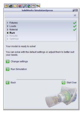
2 Click **Run** to begin the analysis. A status window appears. The stages of the analysis process are displayed with elapsed time.
