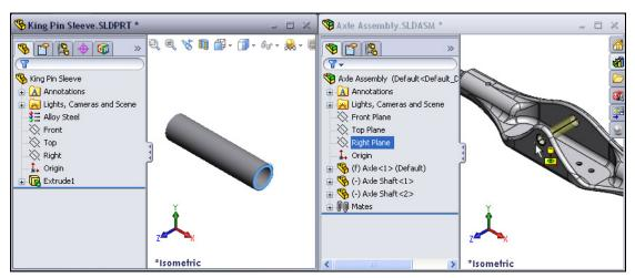
11 Finish the assembly by adding two Socket Set Screws. These set screws are used to keep the axle Shafts from backing out of the axle. The set screws are located in the Mountainboard\ Hardware folder as Socket Set Screw Cup Point\_AM.
