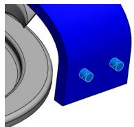
**18** Click the **Offset Entities 1** tool. Type **1mm** for the **Offset Entities** ? distance. Click **OK**. × -12 Parameters Select the top of the other pin, click **Offset Entities** , then 1.000mm Ъ ¥ click 🗹 . Add dimensions Reverse Select chain Bi-directional 1 Make base construction Cap ends Arcs ◯ Lines
