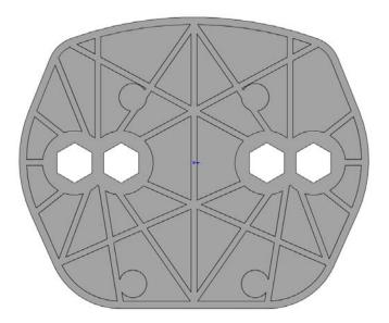
12 If part of a rib is missing, edit the sketch used to create the rib and extend the line into the area where the rib is missing. As an example:
