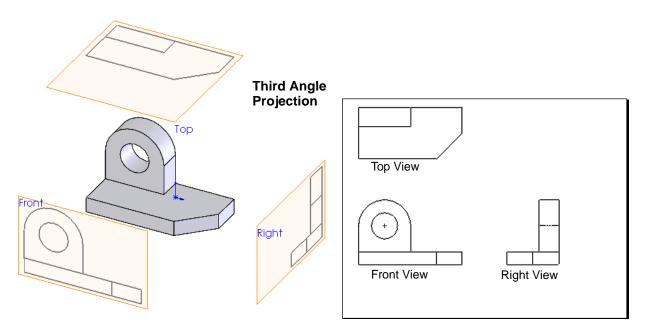
In other parts of the world, the standard is First Angle projection. With First Angle projections, the view is projected on a plane behind the model.
