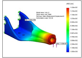
7 To display the result in different units, right-click the Displacement1 plot under the Results folder and select Edit Definition.... Select in from the list in the Units box.
