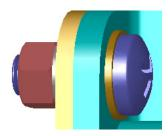
To add these parts to an assembly, select the type of part you want to insert, then drag the Toolbox part into your assembly. As you drag Toolbox parts, they snap to the appropriate surfaces — automatically establishing a mate relationship. In other words, a screw recognizes that it belongs in a hole and snaps to it by default.
