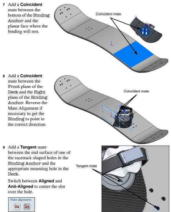
Because the end face of the slot is a cylinder (even thought we only see half of it) we can have two alignments. While we cannot see it, when SolidWorks created the end faces of the slot, it created full cylinders. Part of the cylinder is trimmed away so that we only see the end face.
