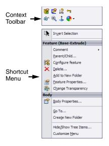
The shortcut menu provides an efficient way to work without continually moving the pointer to the main pull-down menus or the toolbar buttons.
