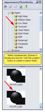
**Note:** Why are we using a different appearance than the part will be made from? With photorealistic rendering, our main concern is what the surface of the model will look like, not the actual material itself. For instance, if we make a part from steel and then apply a layer of paint, it is the paint that we will see, not the steel.
