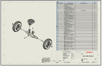
If it is too wide it may cover part of the drawing view. Adjust the column widths by dragging the column borders. When the cursor is over a column border it will change to the pointer shown below.
