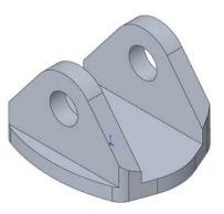
Examine the part. The technique we used was to create three solid bodies that represented the Front, Right and Top view of the combined body.
