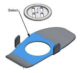
**9** Rotate the model and pick the face shown on the Binding Anchor.
