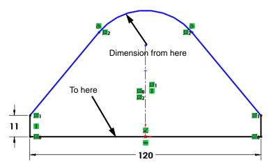
**5** With the dimension selected, drag the end of the extension line from the center of the arc to the arc itself.
