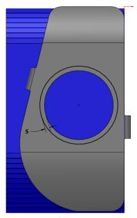
**25** Create an **Extruded Cut** using the end condition **Through All**.
