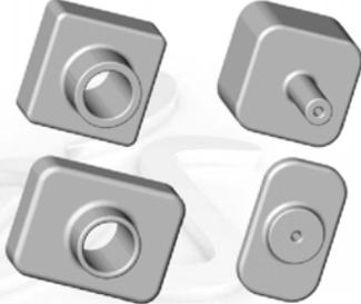
The image displays four 3D models of a square-shaped part with a central hole. Each model represents a different configuration of the part, showing how the dimensions and features change based on the design table settings. The models are arranged in a 2x2 grid, illustrating the variety of configurations possible.
