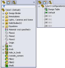
The screenshot shows the Configuration Manager window in SolidWorks. On the left, a tree view lists various configurations: Tutor3 (Default), Design Binder, Annotations, Lights, Camera and Scene, Solid Bodies(1), Equations, Material (not specified), Plane1, Plane2, Plane3, Origin, Box, Knob, Hole\_in\_Knob, Outside\_corners, Fillet3, and Shell1. On the right, a Design Table is visible, showing a table with columns for configuration names and their corresponding design table entries.
