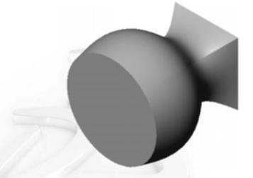
**A Second Loft Feature Creates the Bit of the Chisel:**
