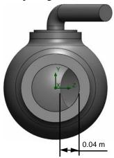
**Note:** SolidWorks Flow Simulation calculates the default minimum gap size and minimum wall thickness using information about the overall model dimensions, the computational domain, and faces on which you specify conditions and goals. However, this information may be insufficient to recognize relatively small gaps and thin model walls. This may cause inaccurate results. In these cases, the Minimum gap size and Minimum wall thickness must be specified manually.
