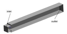
2 Using the Wizard, create the SolidWorks Flow Simulation project for internal water analysis with the **Result resolution** level set to **5** (all other settings are default).
