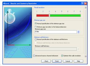
the desired solution accuracy, available CPU time and computer memory. Because this setting has an influence on the number of generated mesh cells, a more accurate solution requires longer CPU time and more computer memory.
