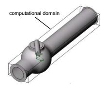
The next step is the specifycation of the boundary conditions. Boundary conditions are used to specify the fluid characteristics at the model inlets and outlets in an internal flow analysis or on model surfaces in an external flow analysis.
