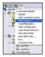
To save time, the Final Default configuration for this section is provided. Configurations allow you to represent more than one version of the part within a single SolidWorks file. For example, by suppressing the features and changing the dimension values of the model, the design can be altered easily without creating another new model.
