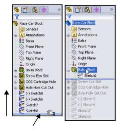
Double-click the Axle Hole Cut Out feature in the Feature Manager. The feature is displayed in blue and Sketch4 is displayed.
