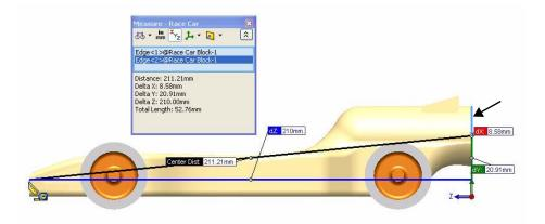
**Note:** The Balsa Block is 223mm x 50mm x 65mm. If you plan to use a fixture to machine your car, you must make sure that your design is no longer that 210mm. Most fixtures have a nose plate that holds the front of the Balsa Block and if your design is too long, it can/will end up breaking the endmill or possible damaging the fixture.
