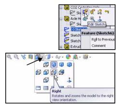
Press the **z** key to Zoom out. Press the **Z** key to Zoom in. Press the **f** key to fit the model to Graphics area.
